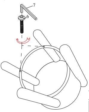
Please leave bolts loosened until all bolts are placed before tightening completely
