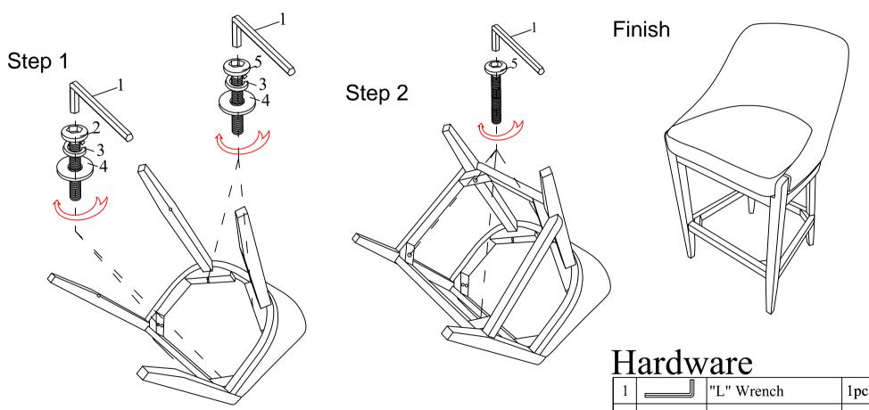
Please leave bolts loosened until all bolts are placed before tightening completely
