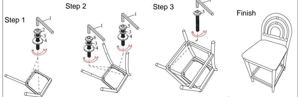
Please leave bolts loosened until all bolts are placed before tightening completely
