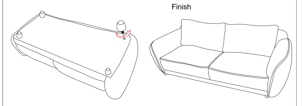
Please leave bolts loosened until all bolts are placed before tightening completely
